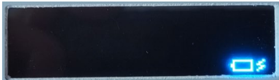
Figure 3: Discharged battery charging symbol.
